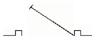
Doorway with Door
